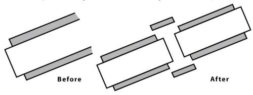
Pro-Tip: Inside corner cut: Note: that when flat, a 45 degree is used, but as the slope increases, the cut angle on the gutter guard DECREASES. Example: on a 4/12 pitch roof, cut at a 43-degree angle. This allows the gutter guard rail to move closer together keeping a good seal while the roof angle decreases.
